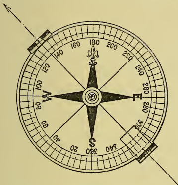
FIG. 119.—Graduation of Prismatic Compass.
